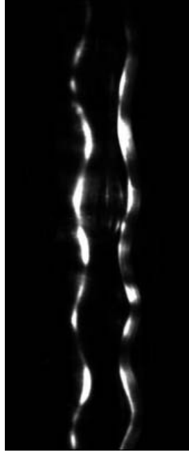
FIGURE 20. Side-view visualization of a symmetric perturbation of the vortices, possibly involving the second radial mode of the elliptic instability. Re = 3600 ; \lambda/a = 3.4 ; a/b = 0.22 .
