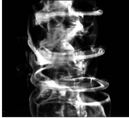
FIGURE 24. Close-up view of the secondary vortices, which are stretched around the final vortex. Re \approx 3000 and \lambda = 3.5 cm.
